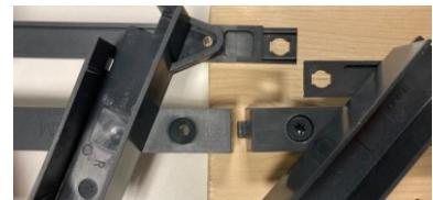
4. Add the following kits by clipping the joint bars and screwing the fixed bars together. Reuse the 7mm spacer at the end.
