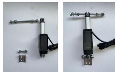
**2.** Mount the bracket and the fork pin on the cylinder. (The cylinder must be retracted, factory setting).
