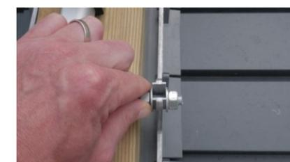
**5.** Lock the nuts on both sides of the forks with a 16 mm spanner. Always keep the blades in the closed position.
