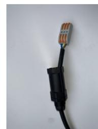
7. Connect the cylinder on the "Motor" side (2 wires: blue and brown) and the general 230V power supply on the "Power supply" side (3 wires: brown=phase, blue=neutral, green/yellow=ground) using the waterproof plugs provided. Inverting the wire colours or reversing the power supply could damage the power supply unit. Do not open the enclosure. Tighten the cable glands to ensure that the connectors are watertight.
