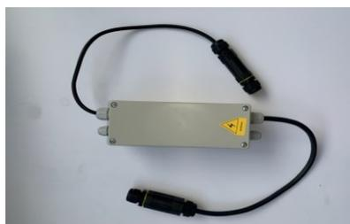
6. Position the power supply unit on the structure or wall of the house so that it remains accessible. For improved durability, it is advisable to position the power supply unit under UV and weather protection. Mechanical protection of the box and cables (sheath, IRL tube...) is also recommended.
