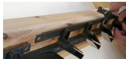
3. Replace with the aluminum stopper rod with the lock facing outwards.
