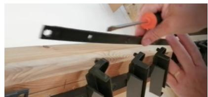
2. Unclip the PVC joint bar from the holders using a screwdriver. Use pliers to remove the locking clips.
